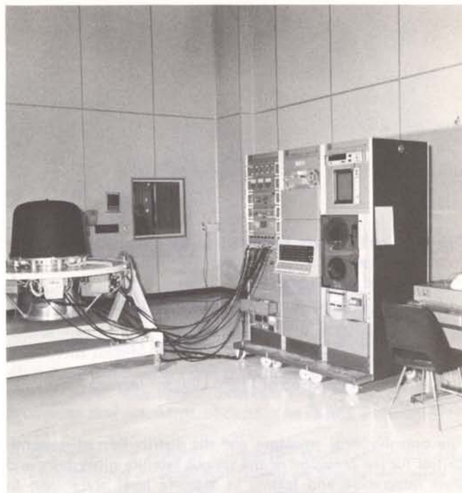
Figure 4 – Integrated central detector package being tested with the payload test equipment at ESTEC.
